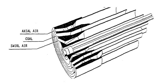
A new generation of multi channel burners has therefore been designed. With special arrangements and constructions of the primary air channels the above mentioned negative effects can be avoided through the creation of a longer and more homogenious internal recirculation zone in the flame (see chapter 3.2.2).
